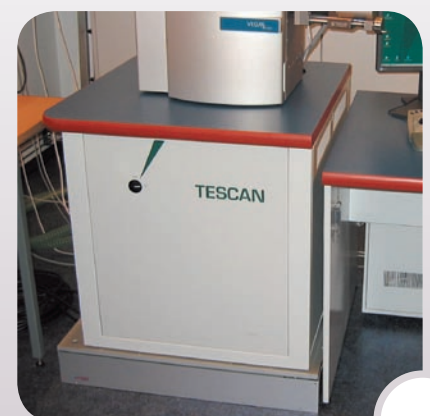
▲ Tescan Vega II XMU SEM on a Halcyonics SW 800-4.0 platform
